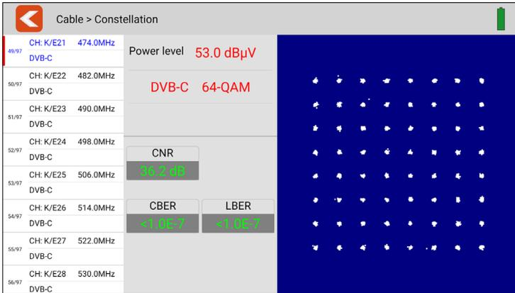
This submenu shows the constellation diagram of the live stream. All frequencies are listed on the left side of the menu. Tap on the display area of the frequency to switch to it.
