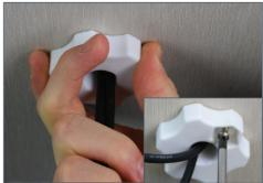
8. From the inside of the vehicle, attach the clamp and turn clockwise onto the thread protruding from the bottom of the antenna. Continue to turn until the clamp is compressing the seal underneath the antenna.
