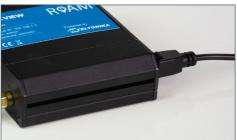
4. Connect the 12V power lead or the 230V PSU and route the lead to your power source.
