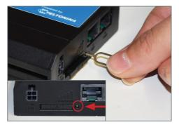
**1.** Use pin to firmly press on SIM eject button. This is located next to the SIM slot. It is not necessary to apply force to the SIM tray itself. This may damage the router.
