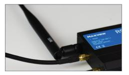
3. Attach the Wi-Fi antenna to the top connector. This is marked 'Wi-FI'. This should be positioned so it is vertical.
