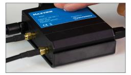
5. Place the router into the mounting bracket. The router can be removed from the bracket at any time to change the SIM card as required.
