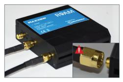
2. Attach the antenna coaxial cables to the bottom 2 connectors. These are marked 'mobile'. Note the order of the cables does not matter.
