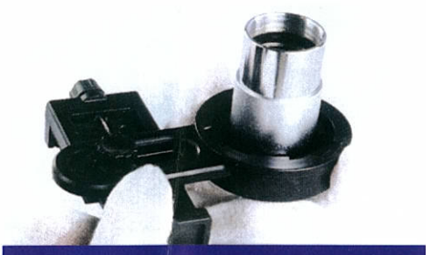
1. Install eyepiece on the mobile phone bracket and lock it up.
